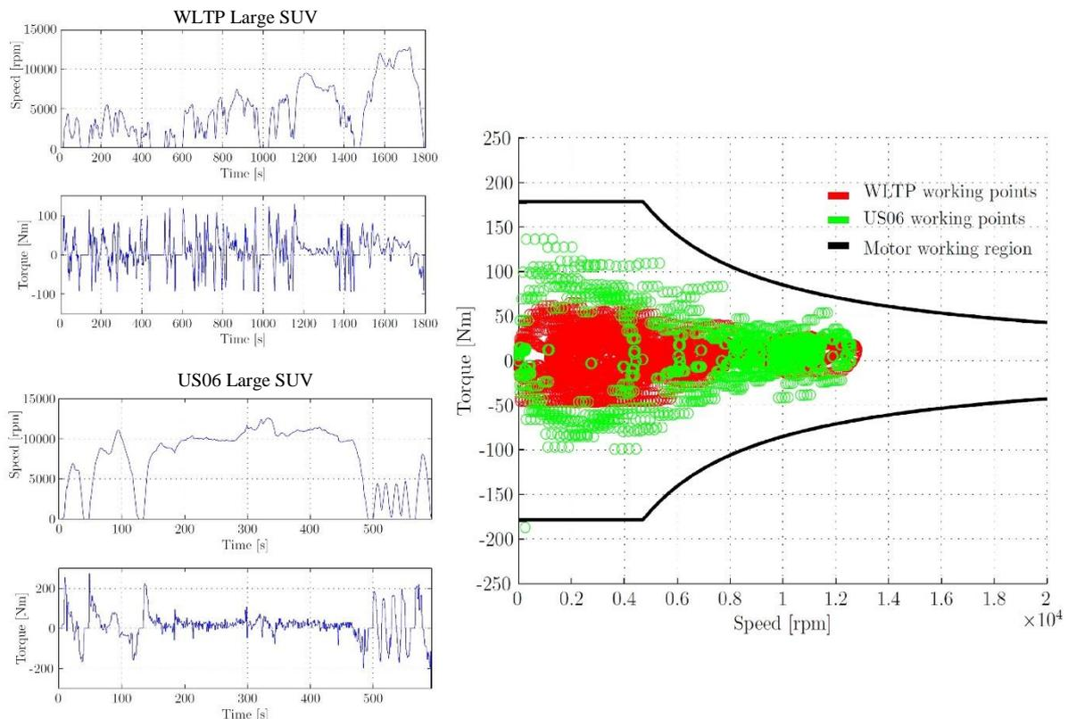
Figure 2: FITGEN electric motor torque vs. rpm envelope and WLTP/US06 operational points for the large SUV vehicle platform with reduction ratio of 1:12.5.
