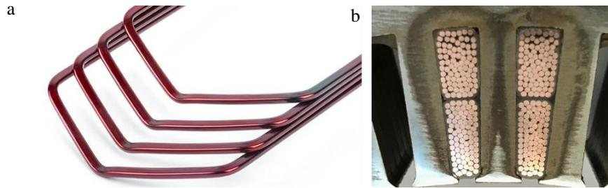
Figure 5: (a) hairpins for HPW (image courtesy of ATOP), (b) cross-section of FLW in the stator (BRUSA proprietary motor).
