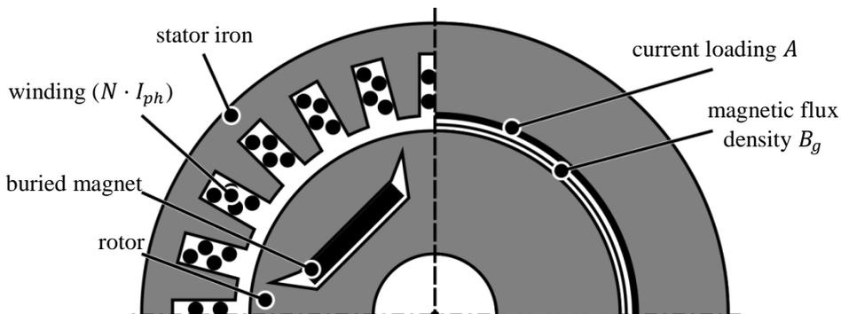
Figure 4: Schematic view of the BPM-SM and the simplification with current loading and flux density in the air gap.
