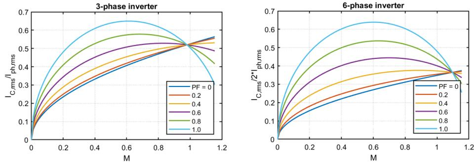
Figure 6: Rms current absorbed by the DC-link capacitor. A) produced by a 3-phase inverter, b) or by 6-phase inverter. Note: the capacitor current is normalized by the phase current of the reference 3-phase motor ( $2I_{ph,rms}$  for the 6-phase case).
