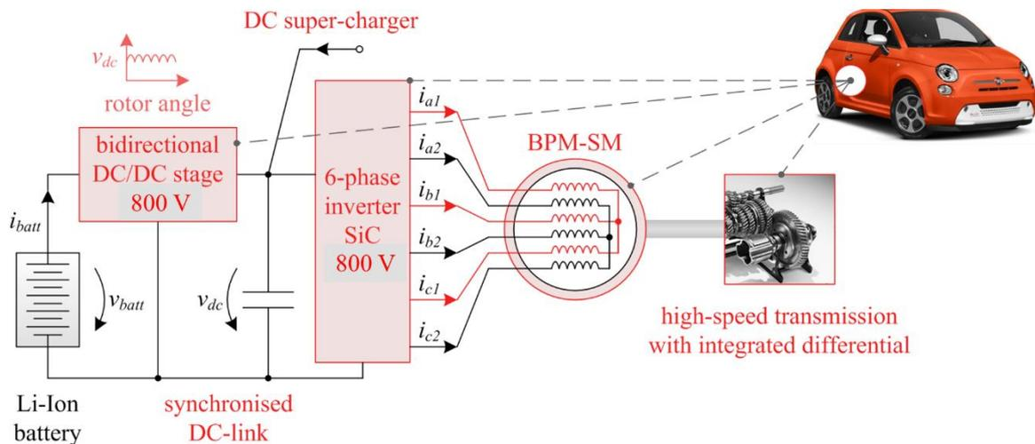
Figure 1: FITGEN e-axle overall architecture (reported graphics are indicative; the final implementation of the e-axle might change).
