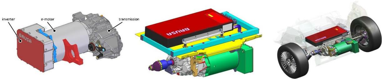
Figure 3: FITGEN inverter-motor-transmission group (left), integration of this group with the DC/DC converter (center) and integration of the full e-axis with the project validator A segment vehicle prototype rear axle (right).
